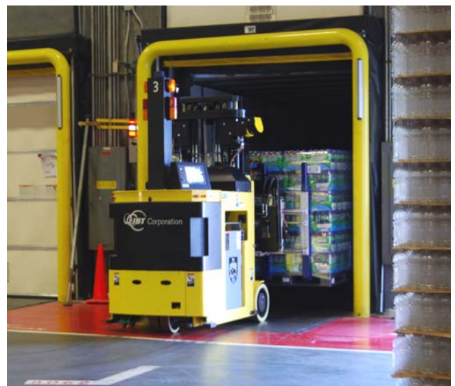
SGV automatically loads a trailer with finished product at the loading docks
